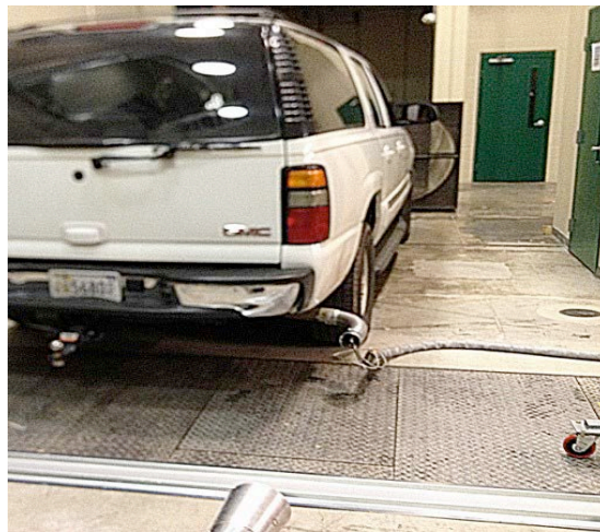
Figure 1: A 2004 Yukon is parked in front of the EDAR unit, above not pictured. EDAR lasers are scanning from above and across the exhaust plume, behind the Yukon. A large fan in front of blows fresh air. The tailpipe probe of the PEMS unit is shown inserted into the tailpipe.
